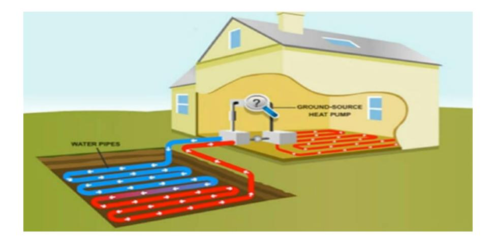
geothermal heat pumps are up to 600 percent more efficient than fossil-fuel powered boilers
